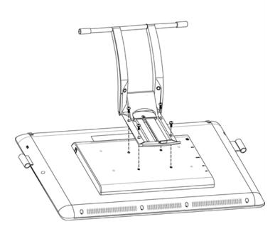
3. Align the four holes in the stand with the mounting holes in the back of the interactive pen display.
